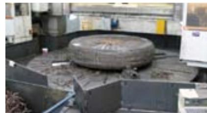
**Forging of NuScale RPV head ingot (diameter 150in, height 30in, weight 142000 lb) by Sheffield Forgemasters and machining of RPV head**
