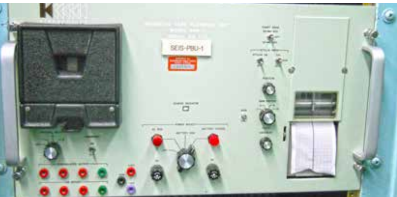
The magnetic tape playback unit in Columbia's Main Control Room provides immediate visual playback capability of recorded ground acceleration data.
